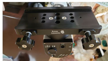
A range of saddles, the top two can do both Vixen and Losmandy. Be careful to ensure the knobs do not protrude and hit the mount at some orientations.
